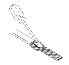
• At the bulge, separate the braid to make an opening.
