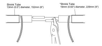
Slide one 13mm (0.5") diameter, 152mm (6") length shrink tube over one of the heater cables. Crimp an insulated splice connector to each bus wire connecting the two heater cables together.
