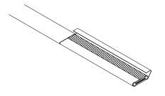
**B** Remove overjacket from heater cable.
