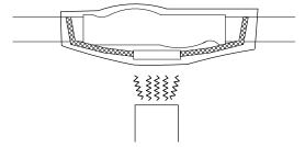
• Center the 16mm (0.63") diameter, 229mm (9") length shrink tube over the splice and braid connection. Shrink with heat gun until completely shrunk. A uniform bead of glue should appear around the ends of the shrink tube.
