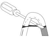
• While bending the heater cable, work it through the braid opening.
