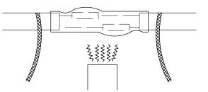
Center the 13mm (0.5") diameter, 152mm (6") length shrink tube over the connectors leaving the braid straps exposed. Shrink with heat gun until completely shrunk. A uniform bead of glue should appear around the ends of the shrink tube.
